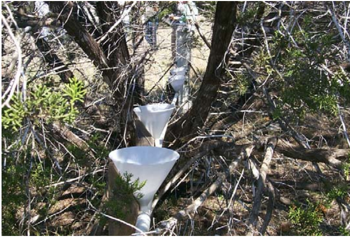
Throughfall funnels and piping system.
